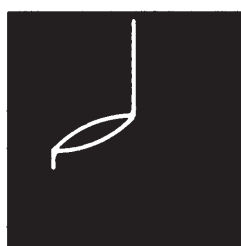
B-E with 1 \mu\text{F} + 680 \Omega
