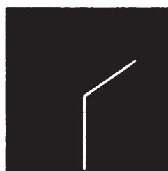
Diode paralleled by 680 \Omega
